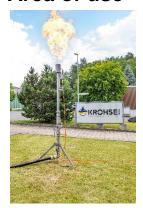
Residual gas quantities should be removed from the area of a blocked, shut-down supply line or a supply line filled with a new medium. For any environmentally conscious corporate philosophy, these should be flared to avoid methane emissions.
